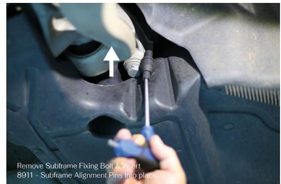
Remove Subframe Fixing Bolt & Insert
